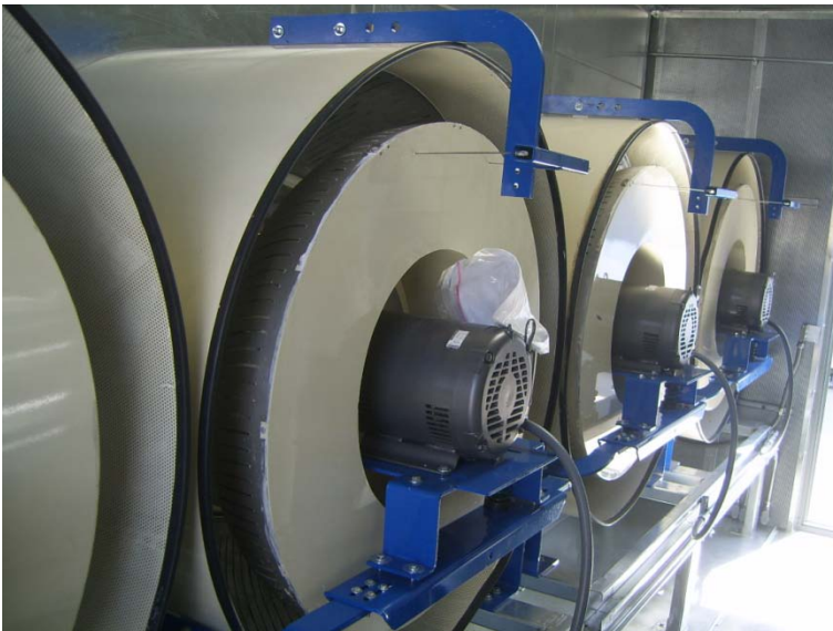
A low/wide aspect ratio 63,000 CFM at 8" SP
